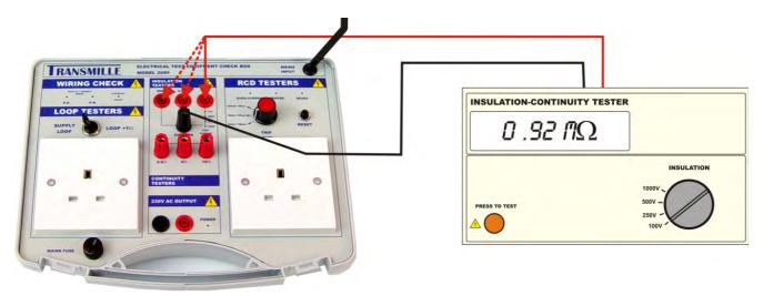
2: Select the lowest test voltage range on the tester, 100V or 250V, and press test button on the tester. Note the corresponding Voltage LED on the 2080 lights. Record result as pass on the check sheet. Check the other test voltage ranges in the same way.
