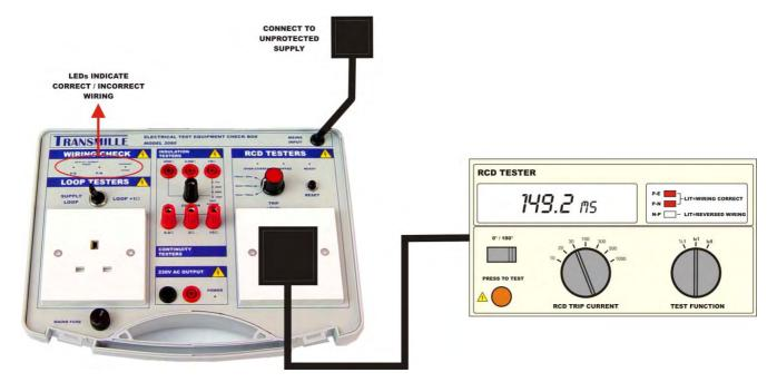
2: Select the 10mA range and the 0° setting if available on the tester, and the 10mA/150ms range on the 2080. Press the reset button on the 2080, wait for the tester to be ready then press test on the tester. The 2080 'tripped' LED will light and the 'Over Current' LED should be off. Record the time displayed on the tester.
